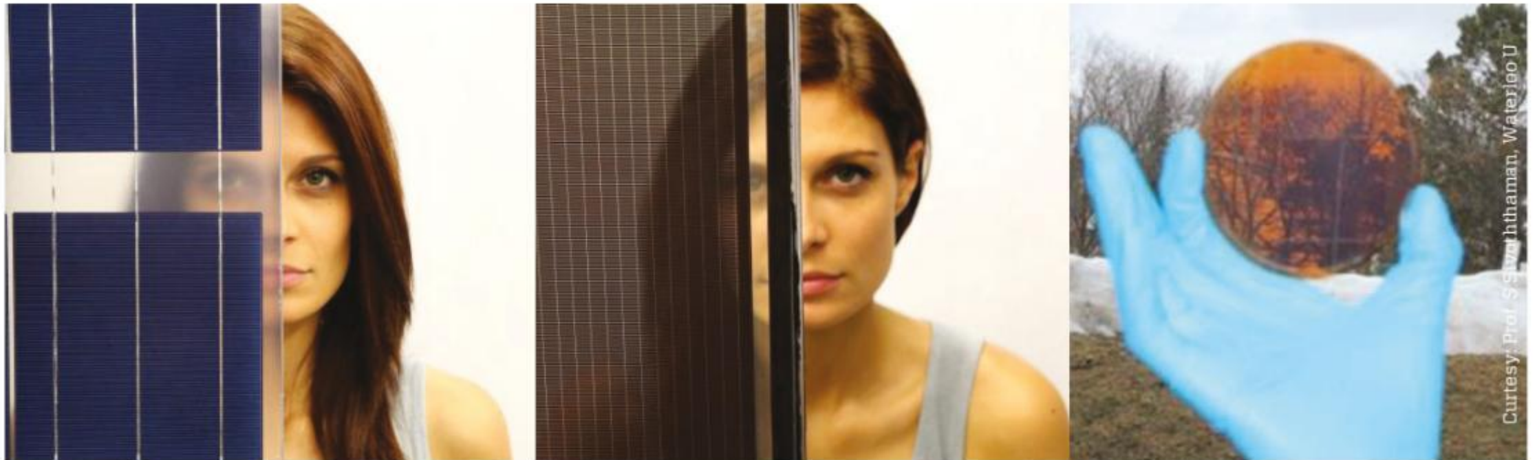
Figure 2.1. Matrix-based STPV windows using: poly-Si opaque spaced PV cells (left), induced-based “see-through” \alpha -Si/ \mu c-Si thin film (centre) and fully transparent \alpha -Si/nc-Si thin film that can be used on intrinsic-based applications (right).
