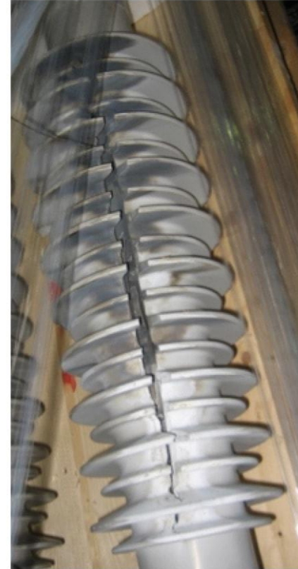
b) Mold-in-place housing split.
