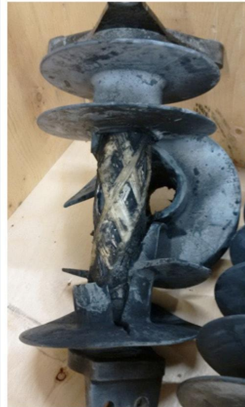
a) Slip-on housing blown off.
