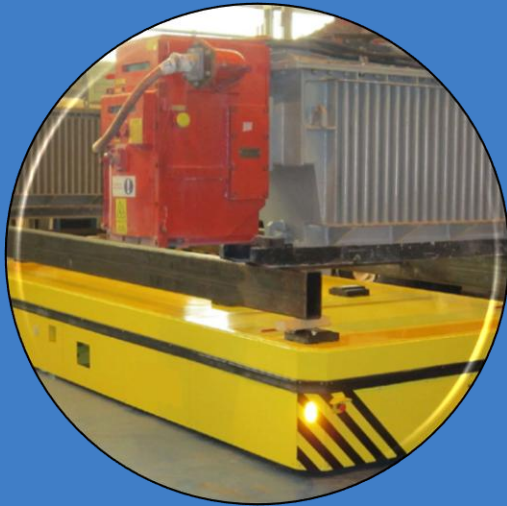
AGV (Automated Guided Vehicle) Fixed routes and predefined paths
